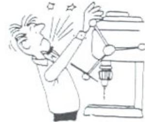
4. Remove adjusting keys and wrenches. Form habit of checking to see that keys and adjusting wrenches is removed before turning it on.
