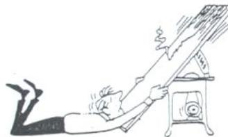
**13.** Secure works. Use clamps or vise to hold works, when practical. It's safer than using your hands and it frees both hands to operate tool.
