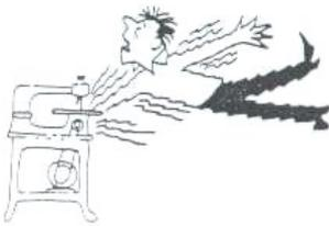
3. Ground all tools. If tool is equipped with three-prong plug, it should be plugged into a three-hole electrical receptacle. If an adapter is used to accommodate a two-prong receptacle, the adapter wire must be attached to a known ground. Never remove the third prong.
